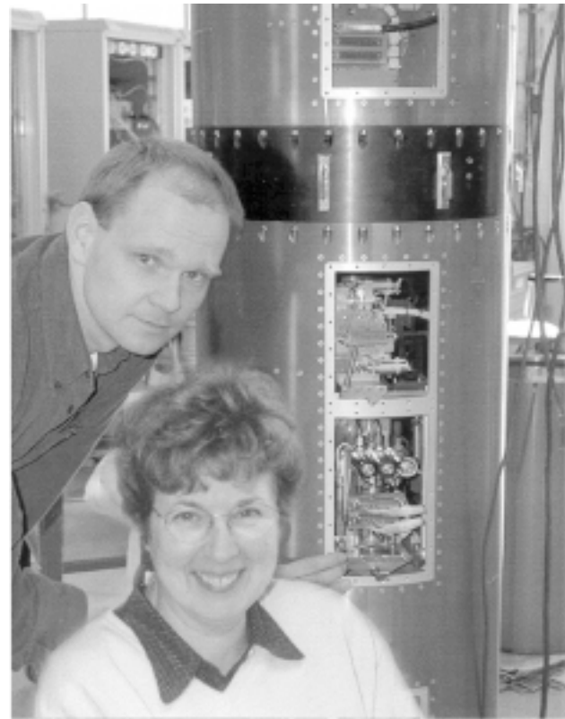
Fig. 4. Brigitte Buchen and Markus Braun in front of a TEXUS rocket. The open windows allow a look at the two late access units for in vivo videomicroscopy and chemical fixation of Chara rhizoids and protonemata.
