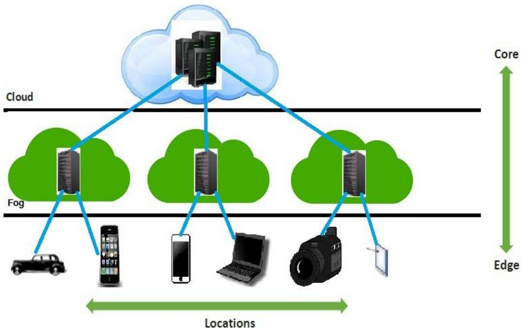
**Figure 1. Fog between Edge and Cloud Computing**
