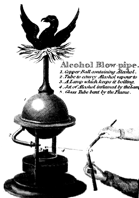
Figure 5: Apparatus for generating gases, and alcohol blowpipe (Mackenzie 1822, plate IX).
