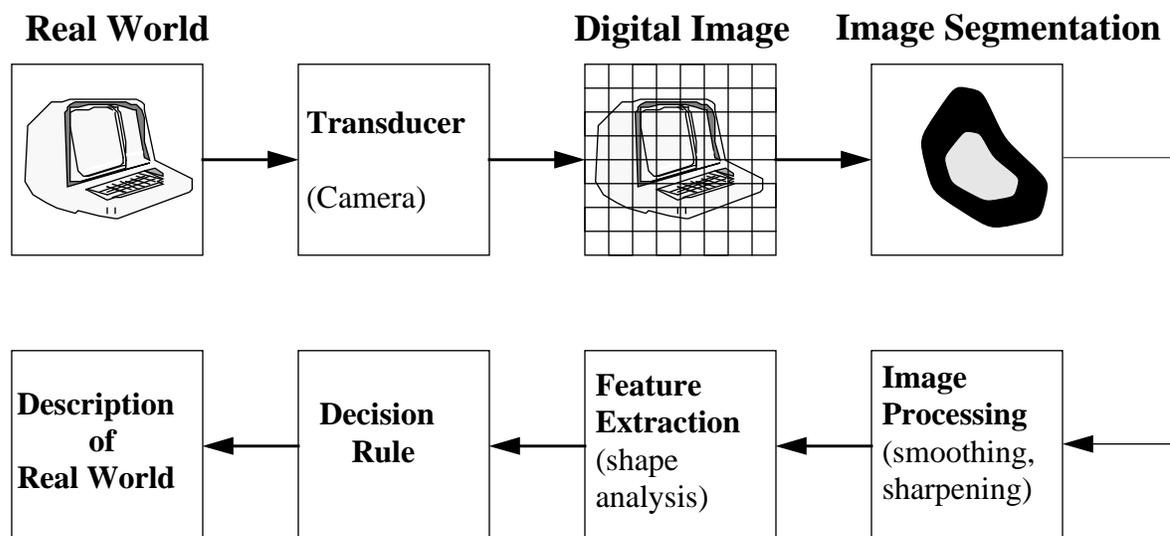
Fig. 3.8 Decomposing the *computer vision* problem into sub-problems.
