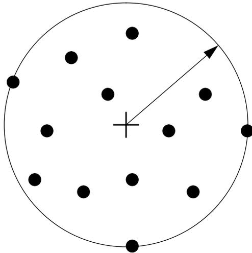
Fig. 2.4 The smallest circle enclosing a set of points.
