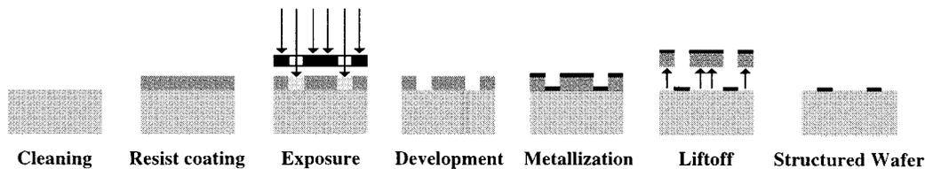
Fig. 3. Process flow of the SAW device fabrication.
