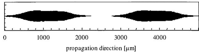
Fig. 2. Geometry of one filter. The meander line through the active taps of both IDTs is depicted.
