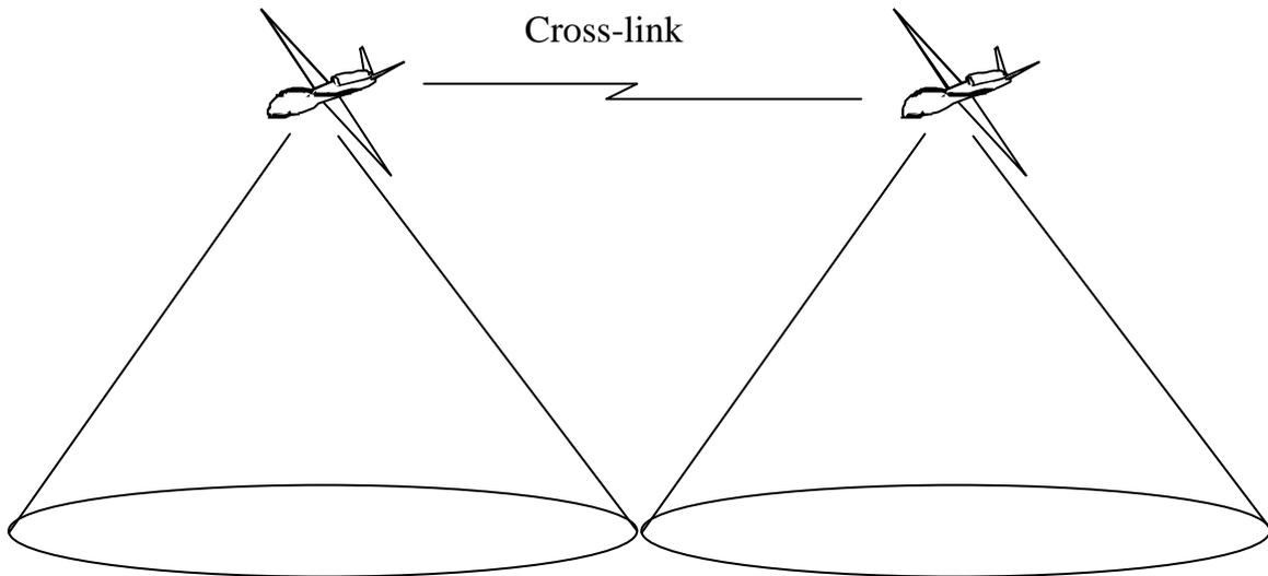
**Figure 3: Increased Coverage by Cross-linking between Airborne Platforms**
