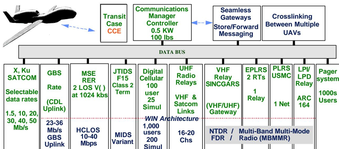
**Figure B-1: Objective Capabilities for US Airborne Communications Node (ACN)<sup>21</sup>**
