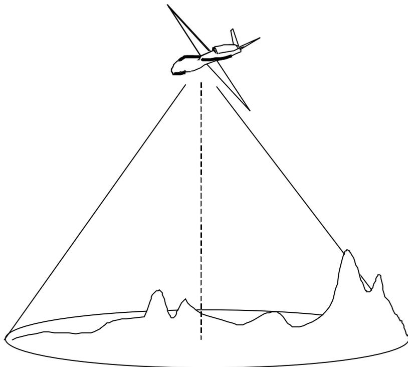
**Figure 5: Effect of Terrain Screening on Propagation Range**
