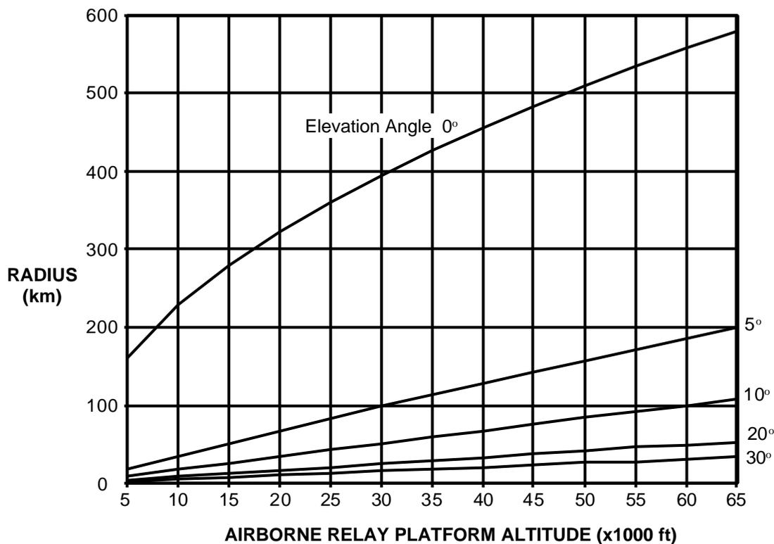
**Figure 6: Airborne Range Extension Radius for Various Antenna Elevation Angles<sup>8</sup>**
