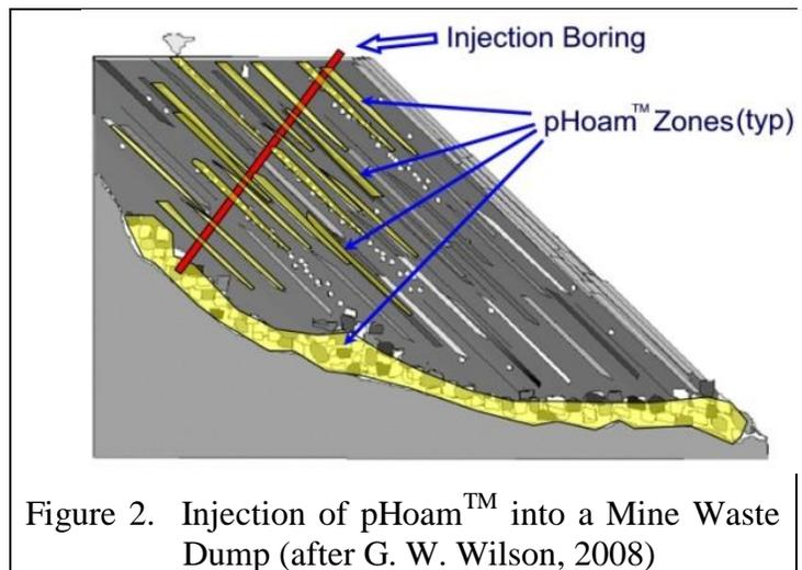
Figure 2. Injection of pHoam™ into a Mine Waste Dump (after G. W. Wilson, 2008)
