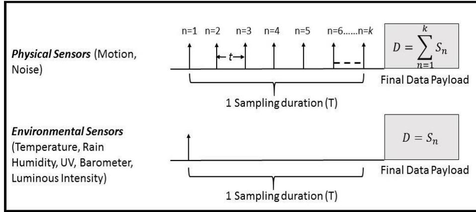
Figure 3. Sensor data acquisition methodology from different sensors.
