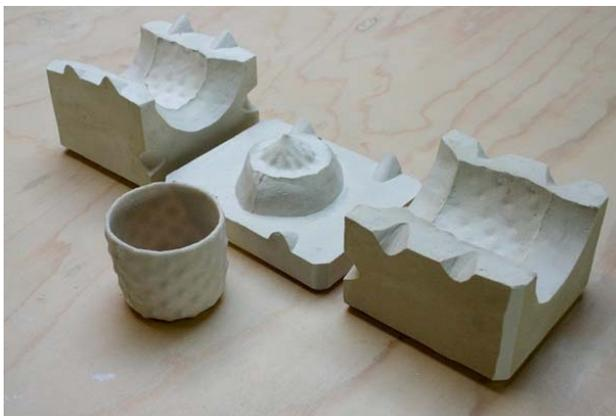
**Figure 10** Intermediate results of the 17<sup>th</sup> century glass reproduction (plaster mold and 3D print).
