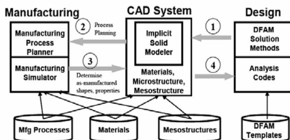
Figure 6 Rosen's DFAM system and method [4].
