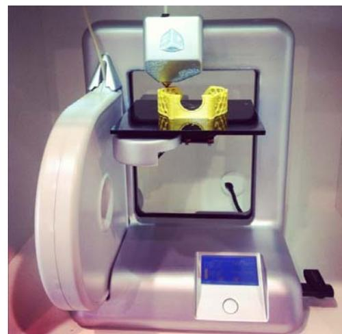
**Figure 3** Low-cost FDM printer (3D systems Cube, \$1200).
